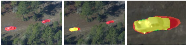
Fig. 6. (at left) result of our moving object detection method, (at the center and at right) the red area represents the result of our method, the yellow area represents the ground truth, and the green area represents the ground truth pixels not detected by our method (the right image corresponds to a zoom on the car on the left part of the center image).
