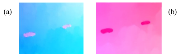
Fig. 2. Dense Optical Flow of images (a) 40-41 and (b) 58-59 of Egtest05 from VIVID. While image (a) is easy to process with the orientation-based segmentation method, image (b) is more challenging due to the coherency of vectors' orientations (represented here by the same hue).
